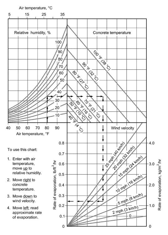
NOTE: If the rate of evaporation exceeds 0.2 lb/ft²/h (1 kg/m²/h) precautions against plastic shrinkage cracking are necessary.
